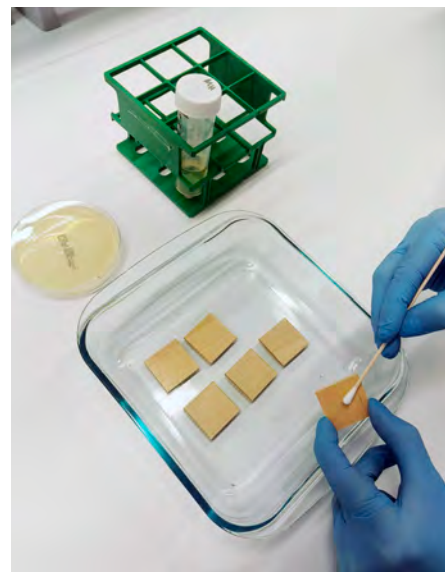
Surface sampling to study the bacterial communities found in the different materials used in a healthcare building
